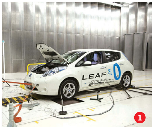
FIG 1: Testing the acoustic characteristics of an electric vehicle involves traditional road noise and wind noise, as well as high frequencies generated by the inverters used to control the power of AC motors through pulse width modulation.
